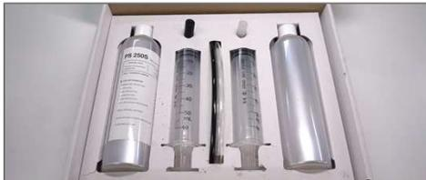
This is the oil changing kit containing 2 syringe, 2 tube, 2 tube connector, 1 oil 1 empty bottle
