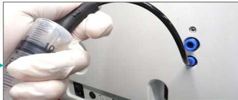
After the tube fully connected slowly pull out the oil out from the unit.
