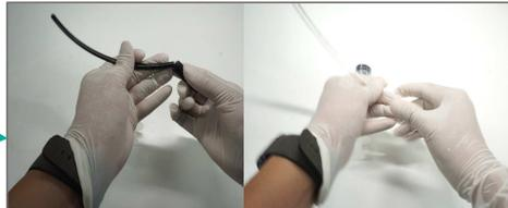
Assemble the rubber with the tube after that connect it to the syringe
