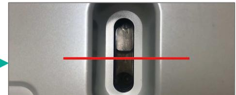
The oil gauge should be slightly higher from the center just like the picture.
