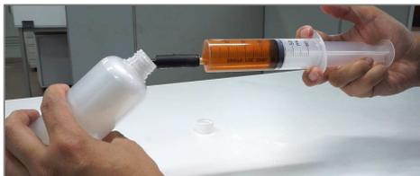
Pick up the black tube syringe and push to put the old oil inside the bottle.
