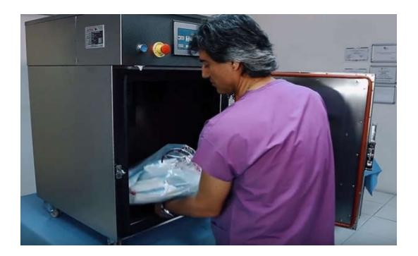
**5-** Once the sterilization bag is inside the chamber, break the ampoule to activate then close sterilizer door. The ampoule is easily broken where the tube narrows at the top.
