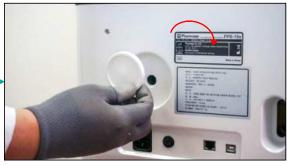
3. Replace it with new HEPA filter by turning clockwise
