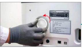
2. Remove the old HEPA filter by turning counterclockwise
