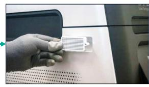
3. Remove the Ozone filter and replace it with new Ozone filter
