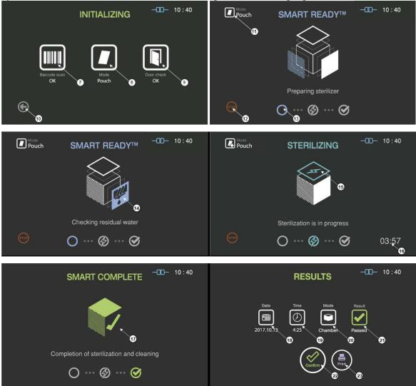
• When the cycle is complete, press Confirm on the Results screen. Should a cycle need to be cancelled before completion, touch the "Stop" button and the screen will ask for a cancellation confirmation. After cycle cancellation is initiated, that process cannot be stopped by the user.
